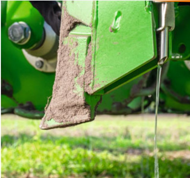
Application of liquid fertiliser on the Primera DMC coulters
