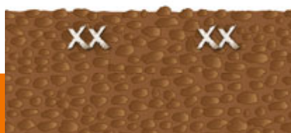
Single-Shoot with 2 applied materials: e.g. seed and fertiliser
