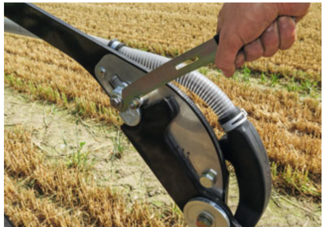
Setting the depth-guided tine coulter
