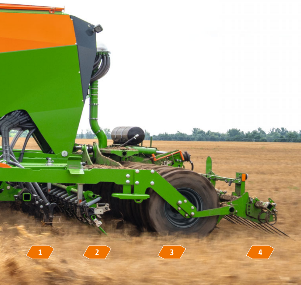
3. Consolidation with the wedge ring roller
