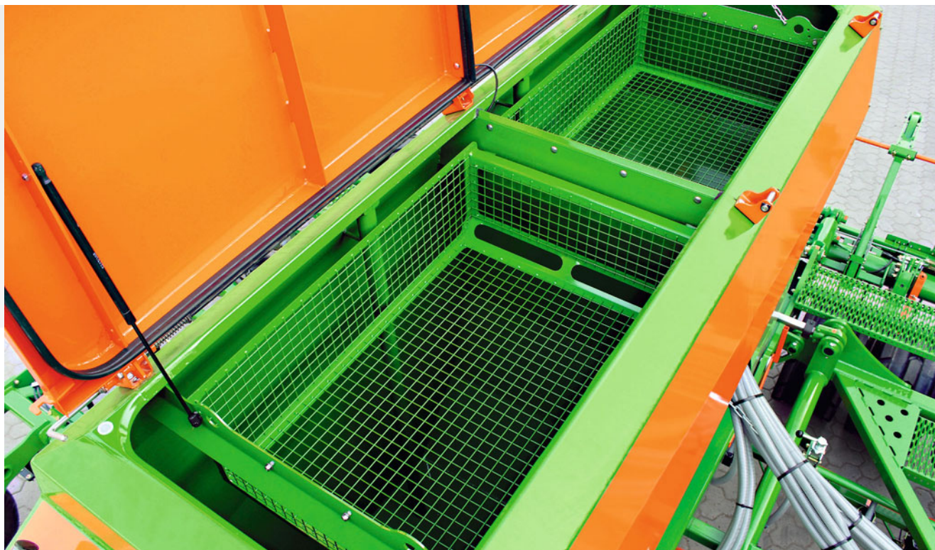
The Cayena 6001-C hopper, divided into two sections in a ratio of 60:40, for 2,400 litres of seed and 1,600 litres of seed or fertiliser, with a pressure-tight sealable lid.
