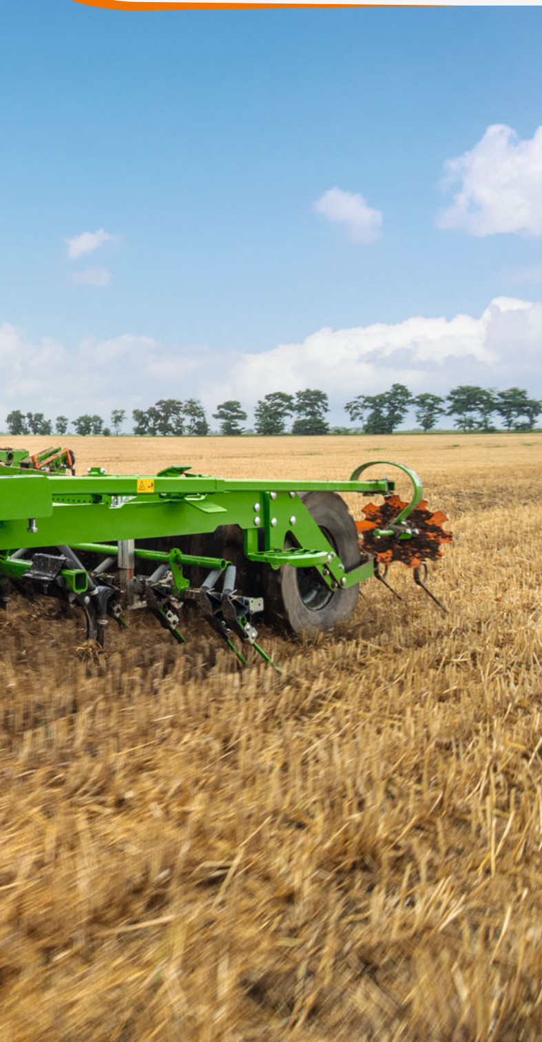
Narrow and tough with the outlet for seed and/or fertiliser – the TineTeC tine coulters
