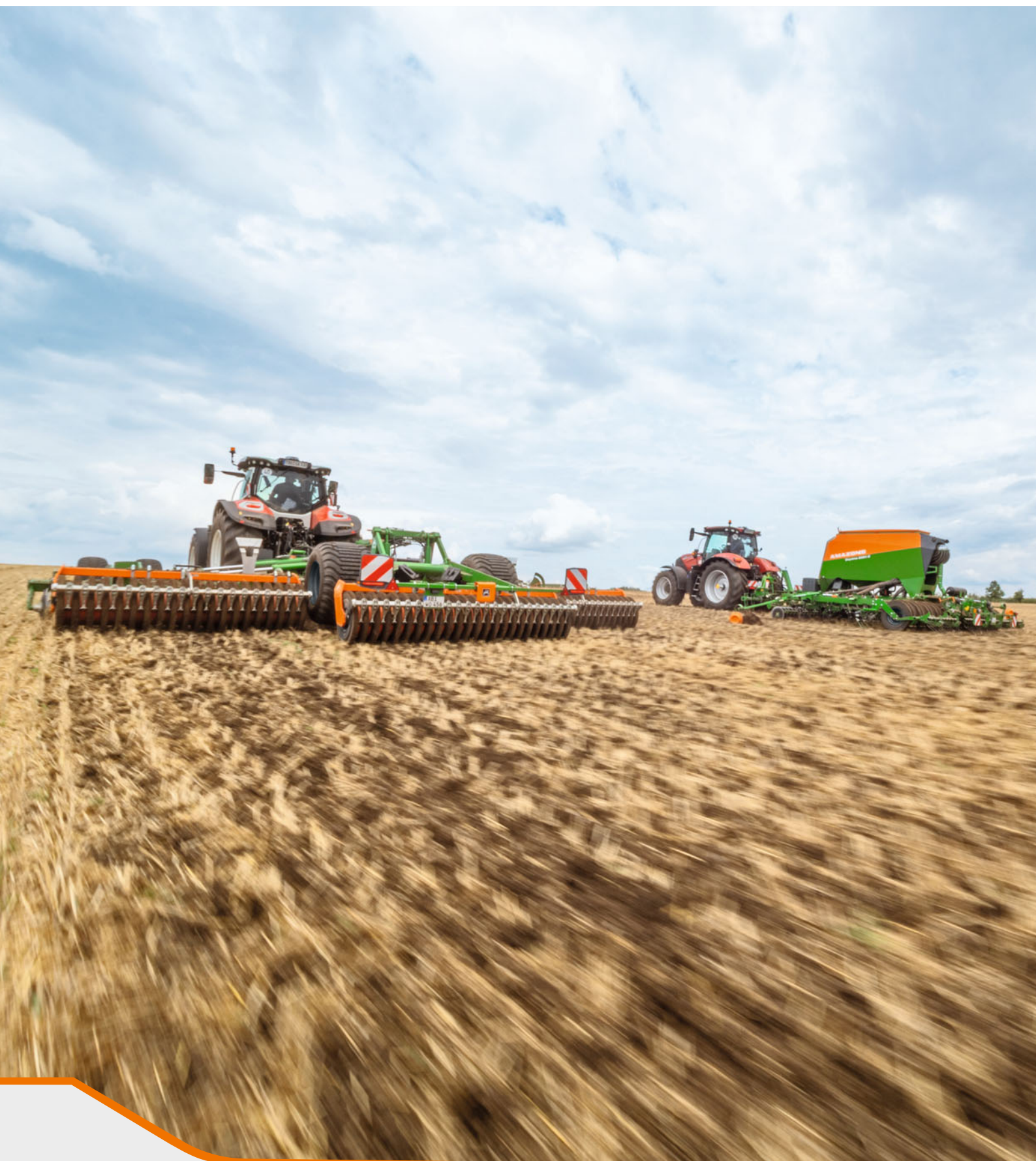
Water-saving mulch sowing with the Cayena, immediately after shallow stubble cultivation with the Catros compact disc harrow from AMAZONE
