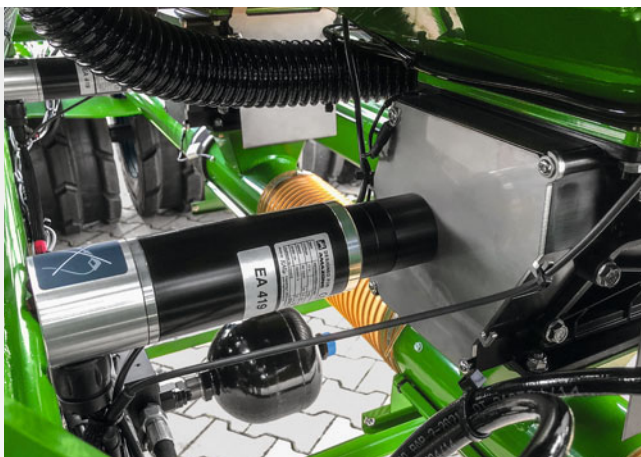
Metering drive below the hopper for the products being transported
