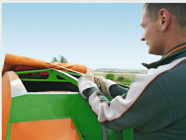
The Cayena 6001 hopper is protected from dust and rainwater by a rollover cover
