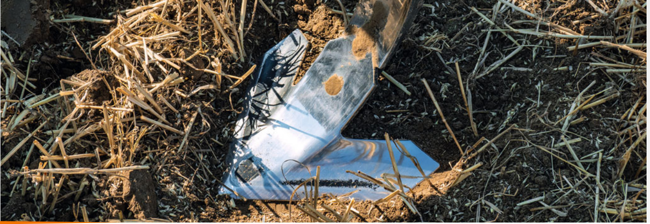
Duckfoot share for minimum working depths of 3 cm
