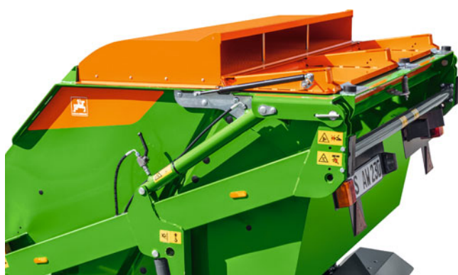
A gas strut dampens the closing movement of the hopper lid after emptying
