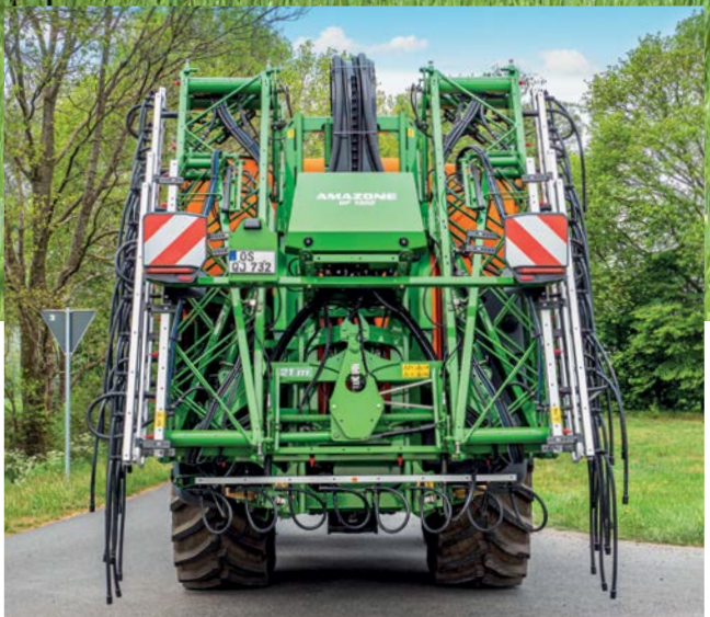
Drag hose with articulated joint
