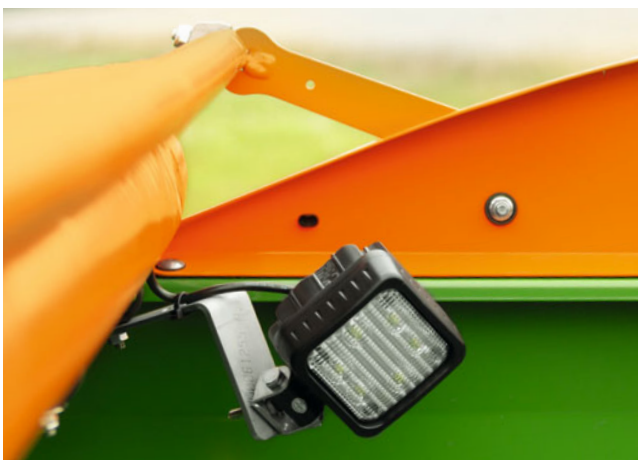
Lighting for the inside of the hopper
