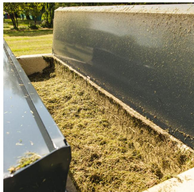
Compacted, cut material in the collection hopper
