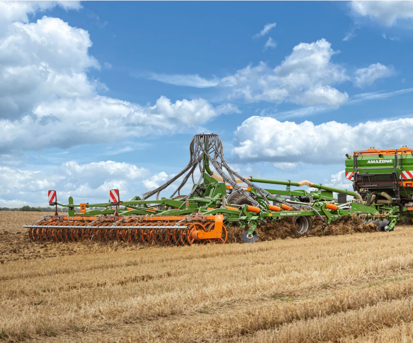
Ceus 7000-2TX Super combined with the XTender 4200 rear hopper for catch crop sowing or fertilisation
