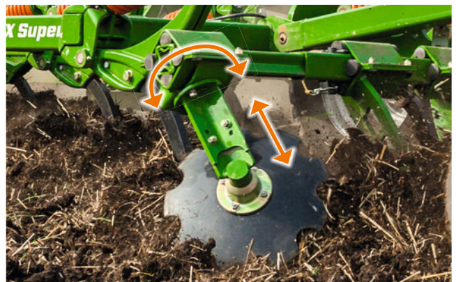
The outer closers – individually adjustable in height and angle
