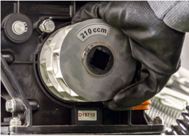
Metering cassettes for different seed types
