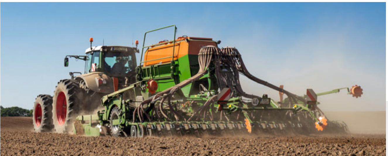
Use of the knife roller to produce a fine soil seedbed when sowing wheat
