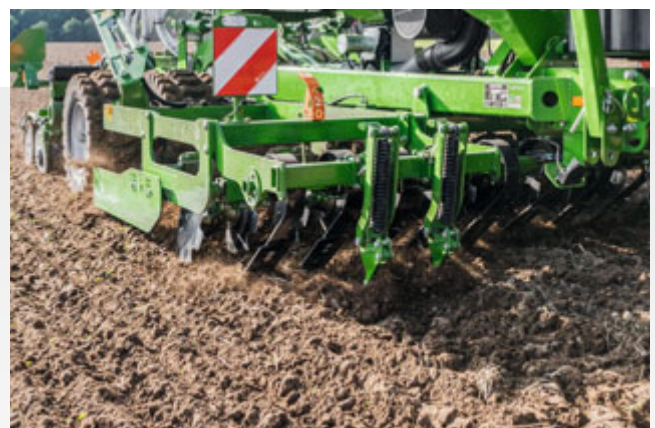
Combination of Crushboard and tractor wheel mark eradicators
