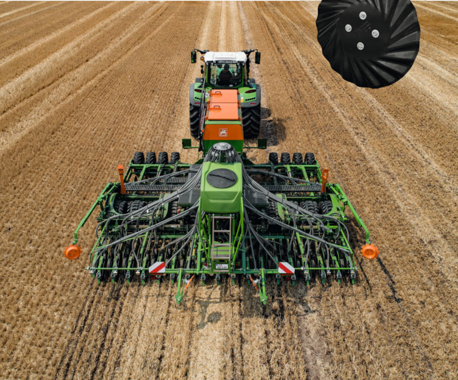
Minimal, water-conserving soil tillage in strips with the Minimum TillDisc cutting disc
