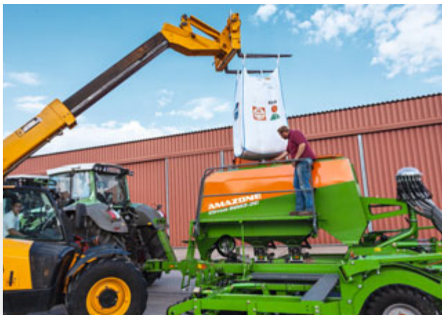
The large hopper opening makes for very convenient filling of the hopper.
