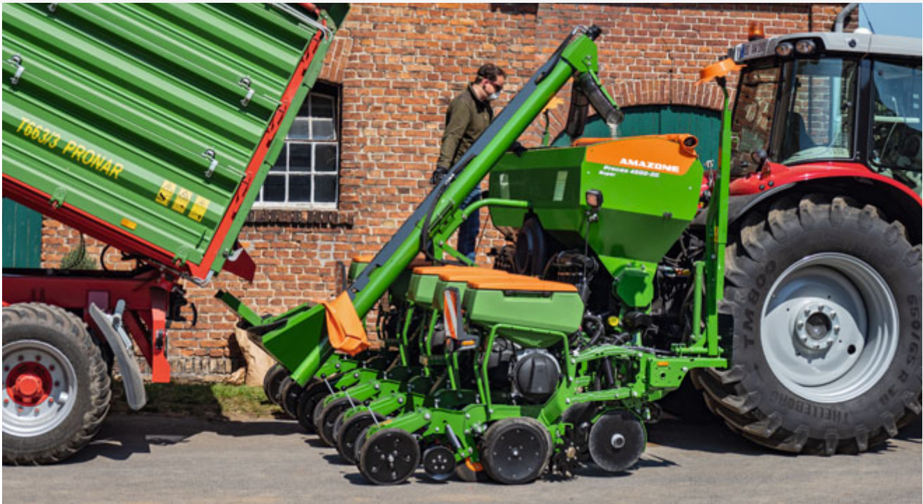
The optional filling auger facilitates convenient filling of the fertiliser hopper
