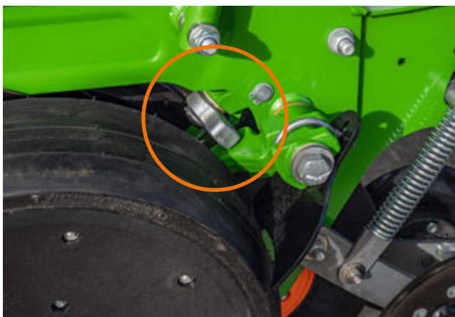
The measuring pin registers changes in the contact force on varying soils. The ISOBUS-controlled SmartForce system then automatically evens out these fluctuations. As a result, the placement depth remains the same under all soil conditions.
