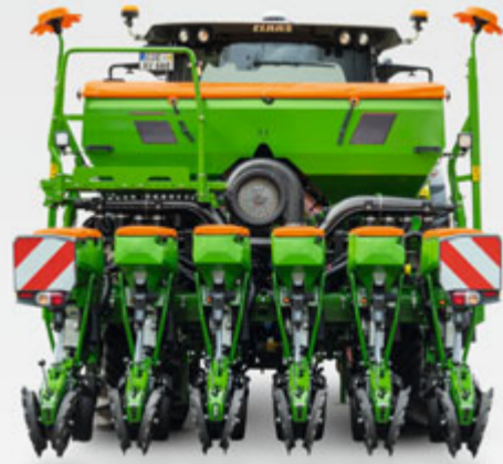
The Precea 4500-2CC with variable telescopic frame set for the narrower working width
