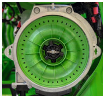
Singling disc in place while stationary
