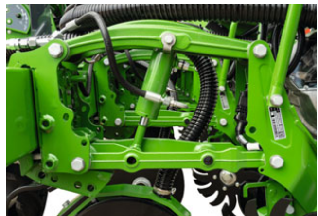
The coulters pressure is automatically adjusted via the hydraulic cylinder
