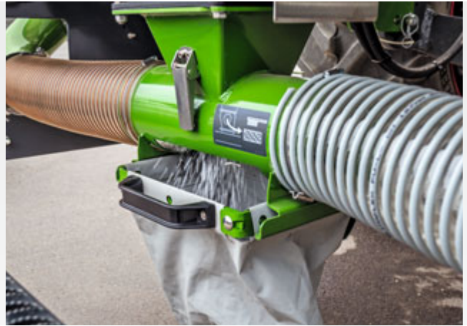
The calibration bag can easily be suspended under the metering unit
