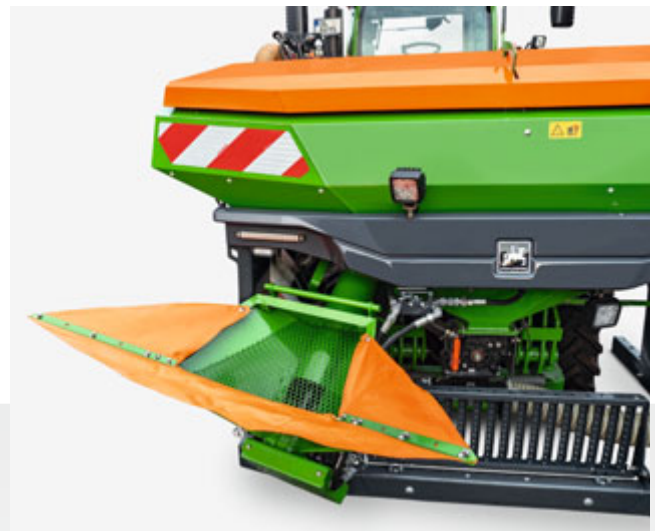
A filling auger with a folding reception hopper is available as an option. This allows easy filling direct from the trailer. The filling auger is securely closed with a lid in the transport position.
