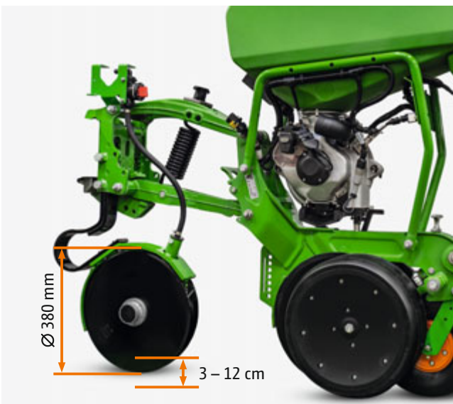
The FerTeC Twin double disc fertiliser coulters with leaf spring overload protection The placement depth is adjustable between 3 – 12 cm, and the maximum coulters pressure is 80 kg
