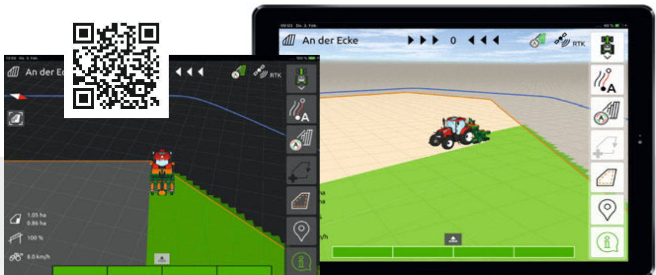
Alternative map views with AmaTron Twin – clear display of the machine and its part-width sections, as well as buttons on the right hand side of the mobile device.
