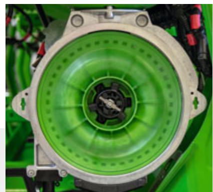
Singling disc in operation (without lid)
