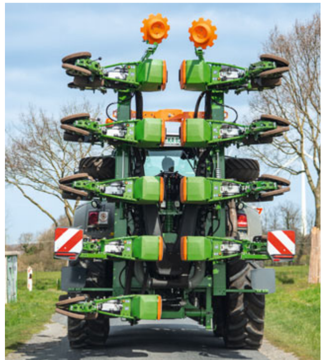
The Precea 6000-2FCC with 9 rows folded for road transport
