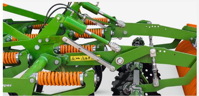
Manual setting of the levelling unit using a holed quadrant raster on rigid machines.
