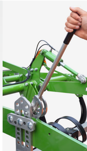
Manual setting of the levelling unit using a holed quadrant raster on rigid machines.
