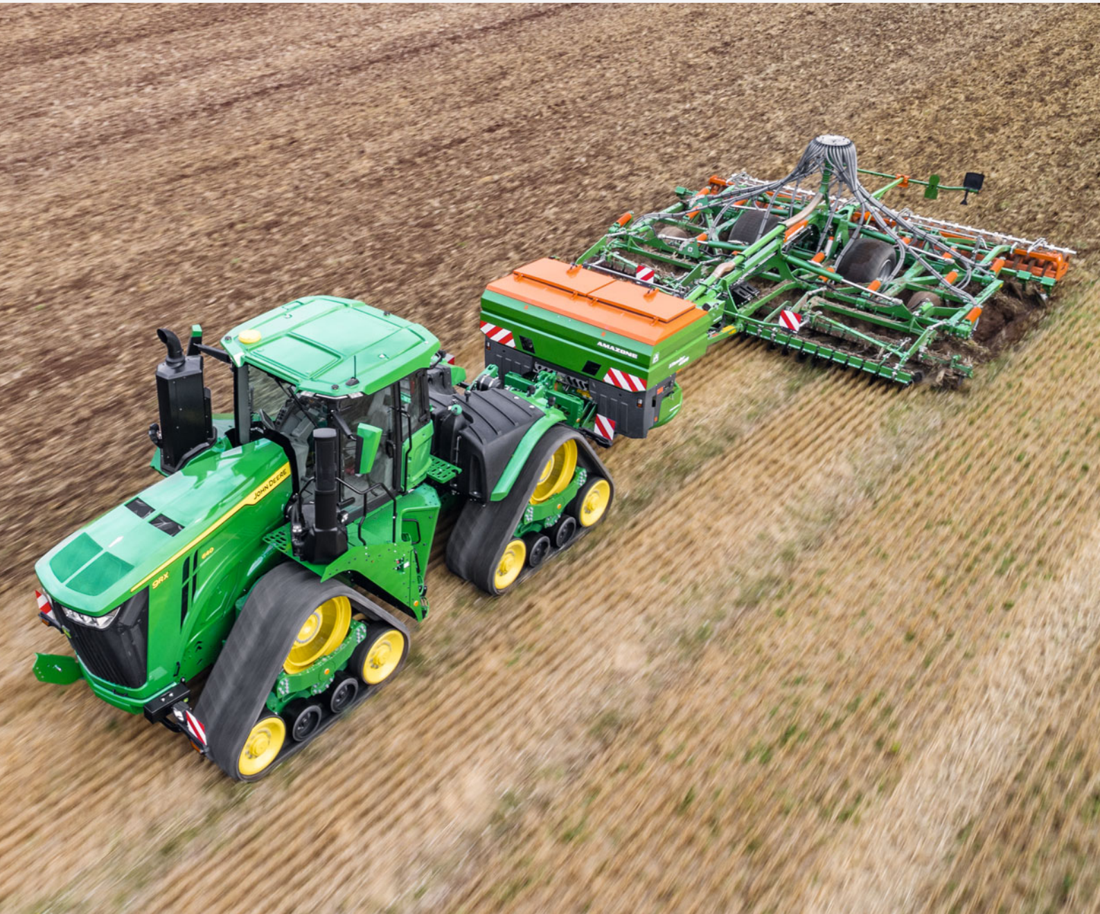
XTender 4200 with a capacity of 4,200 l
