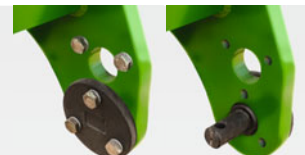
Cenius Special: C-Mix tines with shear bolt overload safety device and WW angle profile roller
