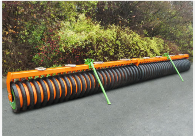
❗ "Due to the bolted clamps, the roller can quite easily be removed for wet conditions or for leaving a coarse 'autumn furrow'." (traction – working test AMAZONE Cenius 5003-2TX Super · 3/2016)
