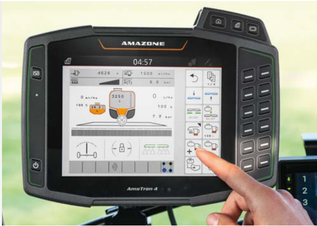
Activation of DirectInject in the AmaTron 4 terminal
