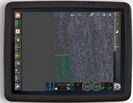
Processing of the spot application map in the ISOBUS terminal
