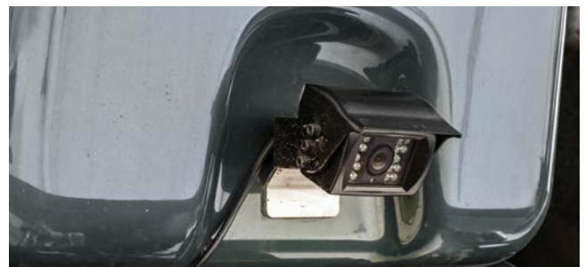
Reversing camera on the rear of the Pantera
