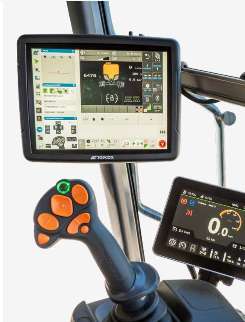
Twin-terminal solution with the TopCon X35 ISOBUS terminal and AmaDrive 7.0 vehicle terminal as well as the AmaPilot + multi-function joystick
