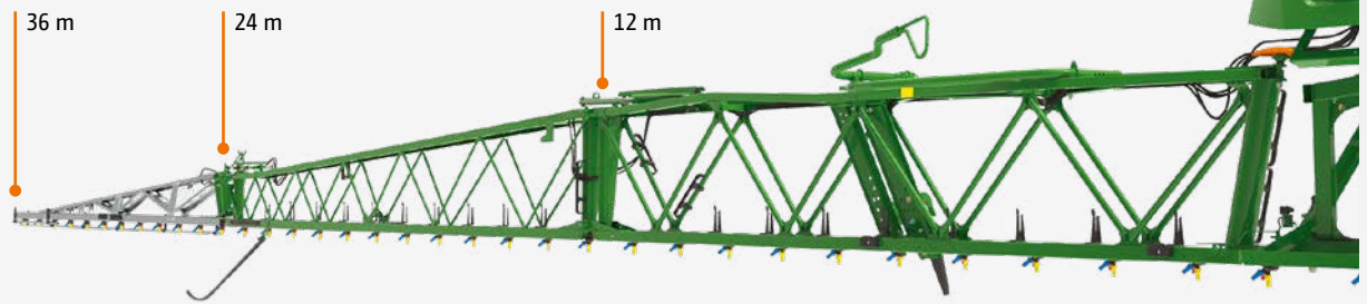
Super-L3 boom with a width of 36 m, folds down to 24 m and 12 m
