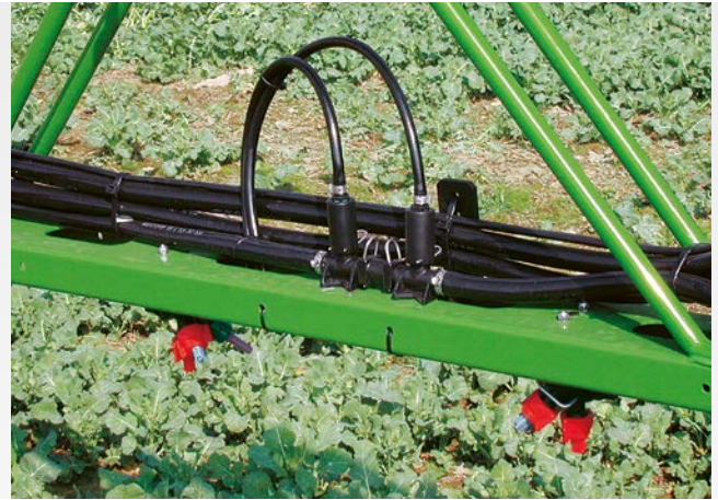
DUS pressure recirculation system
