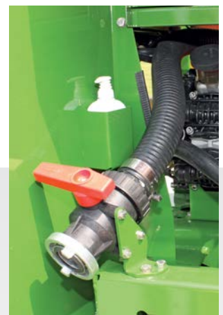
Filling using pressure (C or Camlok coupling)
