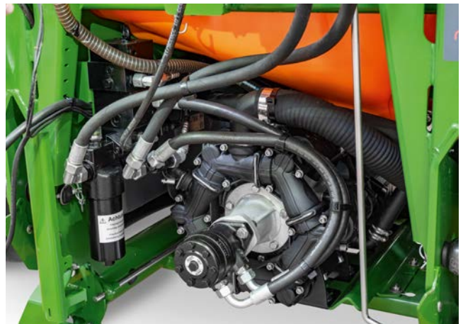
Hydraulic pump drive for the 300 l/min pump on the UF 02
