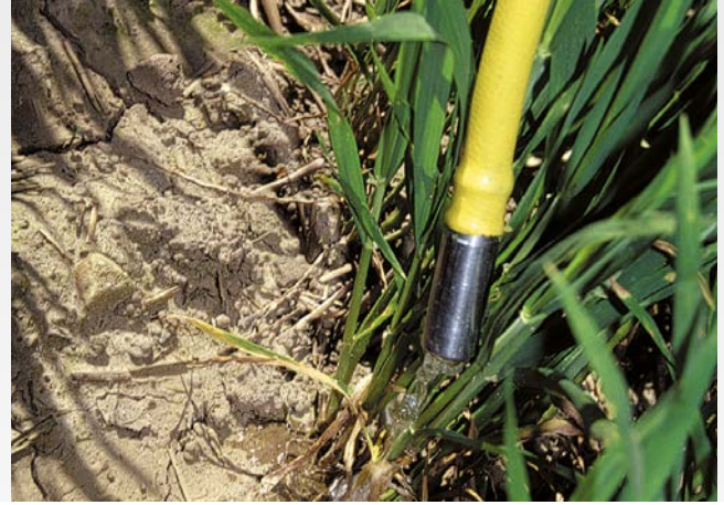
Stainless steel weights on the drag hose
