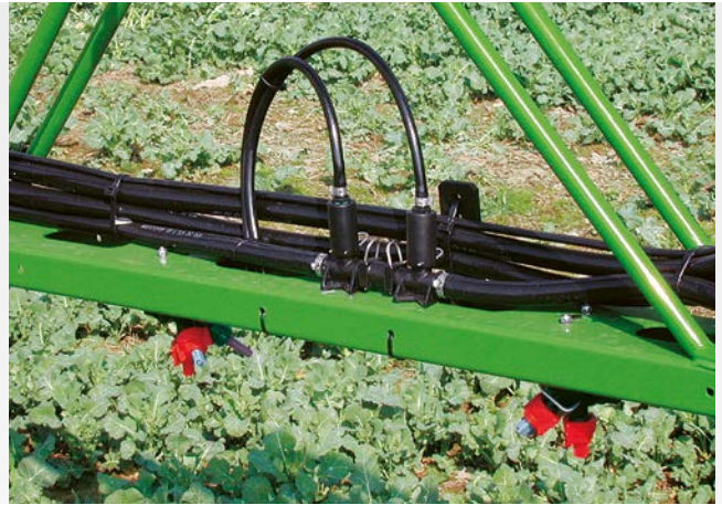
DUS pressure recirculation system
