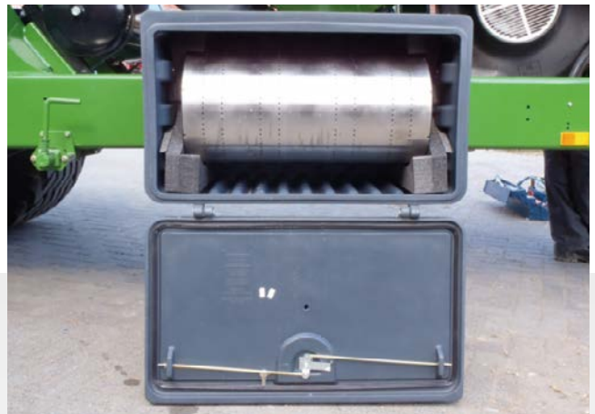
Tool box for an additional metering drum
