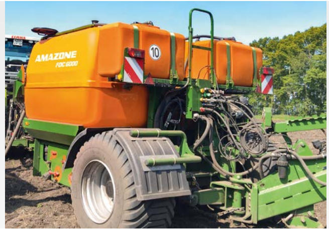
Two 300 l fresh water tanks
