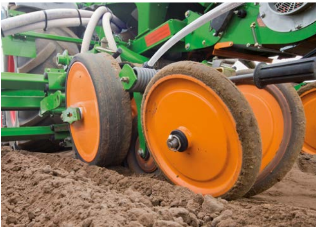
Carrying rollers and furrow closing with Super-V press rollers
