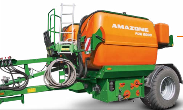
FDC 6000 Additional pulling power requirement of 50 hp
