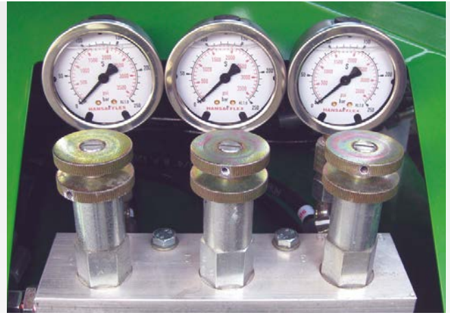
Manual pressure adjustment for the EDX 9000-TC
