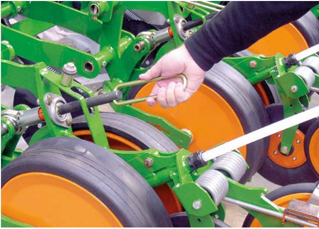
Depth adjustment via a spindle
