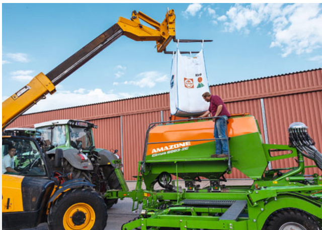
The large hopper opening allows very convenient filling of the hopper
