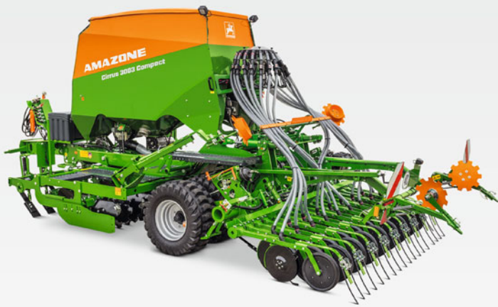
Cirrus 3003 Compact with TwinTeC + double disc coulters
