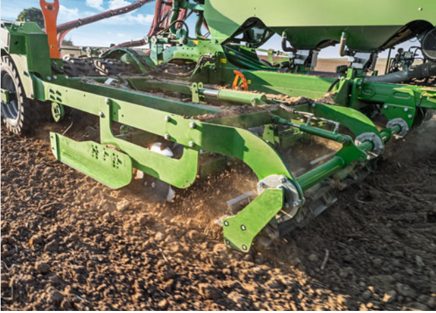
The knife roller as an aggressive front tool for the Cirrus 6003-2
