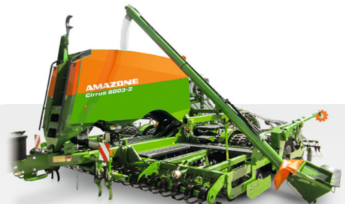
The large hopper opening allows very convenient filling of the hopper
