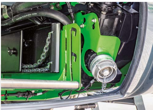
✓ Bowser fill port in the storage compartment with automatic fill stop
