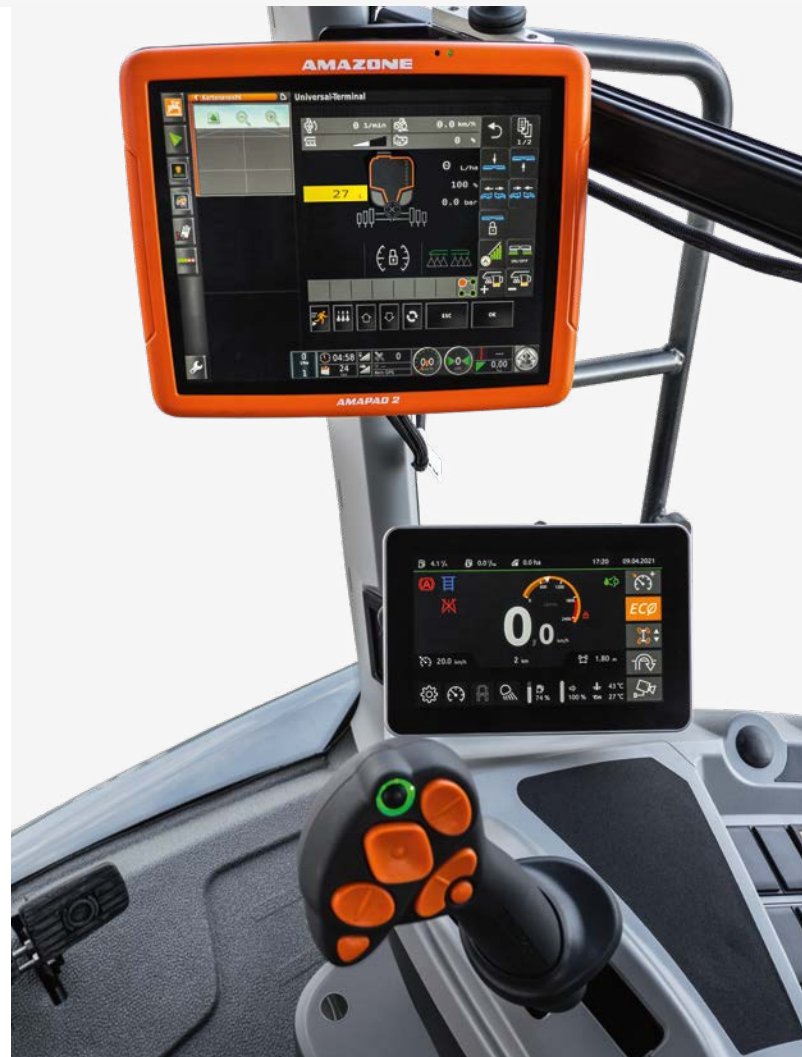
Twin terminal solution with the AmaPad 2 ISOBUS terminal and AmaDrive 7.0 vehicle terminal as well as the AmaPilot+ multi-function joystick
