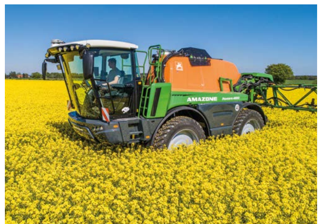
High ground clearance for minimisation of crop damage
