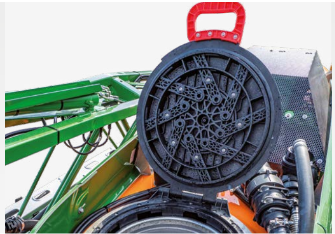
Securely closing tank dome cover
