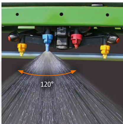
AmaSelect electric individual nozzle control with quad nozzle body and 50 cm and 25 cm nozzle spacing
