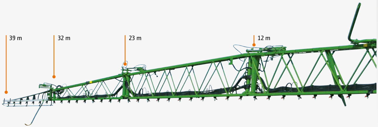
39 m Super-L2 boom, folds down to 32 m, 23 m and 12 m
