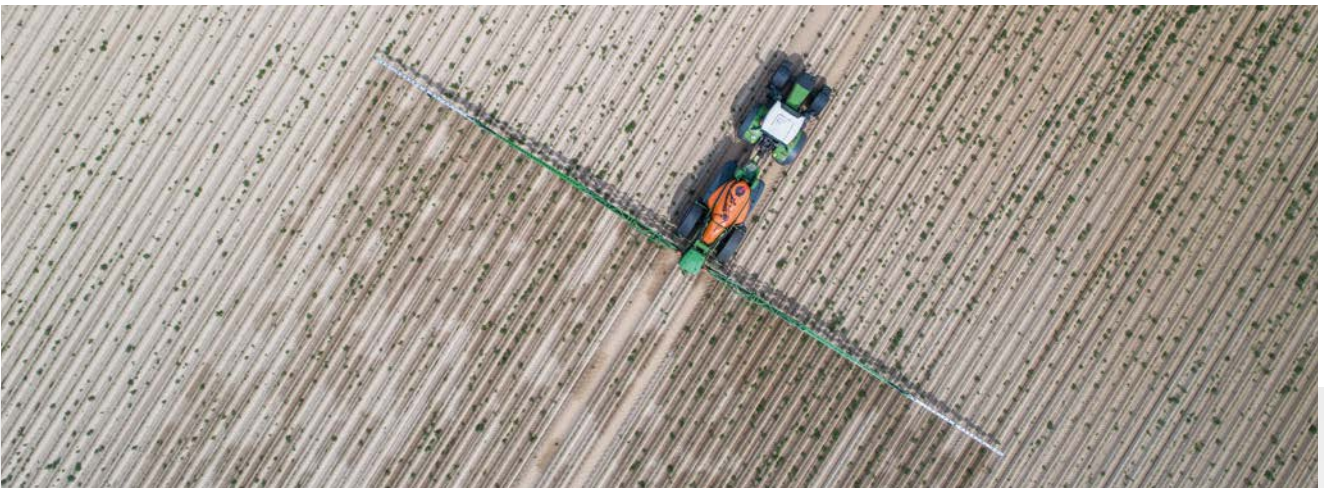
State-of-the-art crop protection technology in use: targeted treatment of volunteer potatoes in a carrot crop on the basis of a spot application map with a standard UX 5201 Super trailed sprayer
