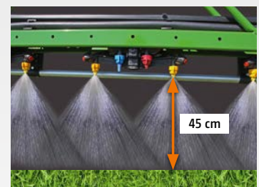
80° nozzles: 25 cm nozzle spacing
