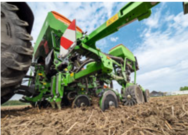
Precea in work with tractor wheel mark eradicators
