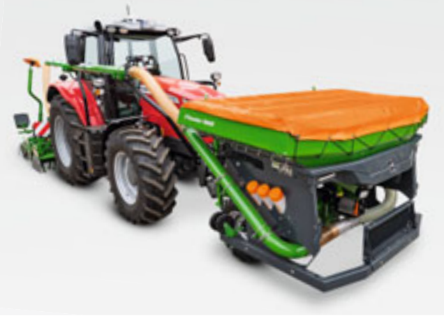
FTender 1600 with open conveyor system and roll-over hopper cover
