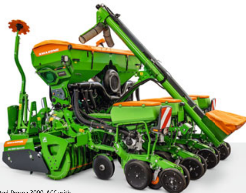
Harrow-mounted Precea 3000-ACC with KG 3001 Special rotary cultivator
