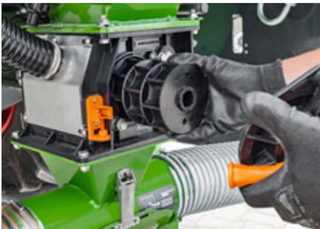
Simple exchange of the metering cassettes on the FTender
