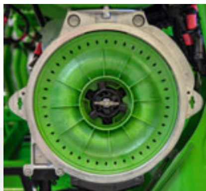
Singling disc in place while stationary
