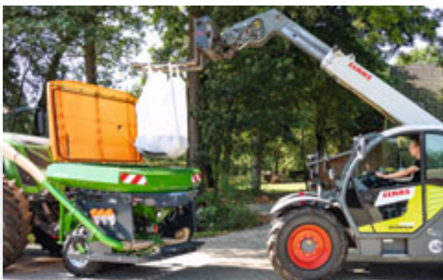
Large opening of 1.1 m x 2.2 m for quick and easy filling of the FTender
