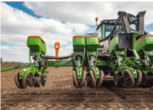
Large row spacing for creating a tramline with an offset unit
