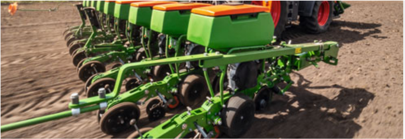
Seed hoppers located above the singling system
