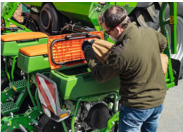
The seed hoppers are easily accessible and facilitate one handed operation
