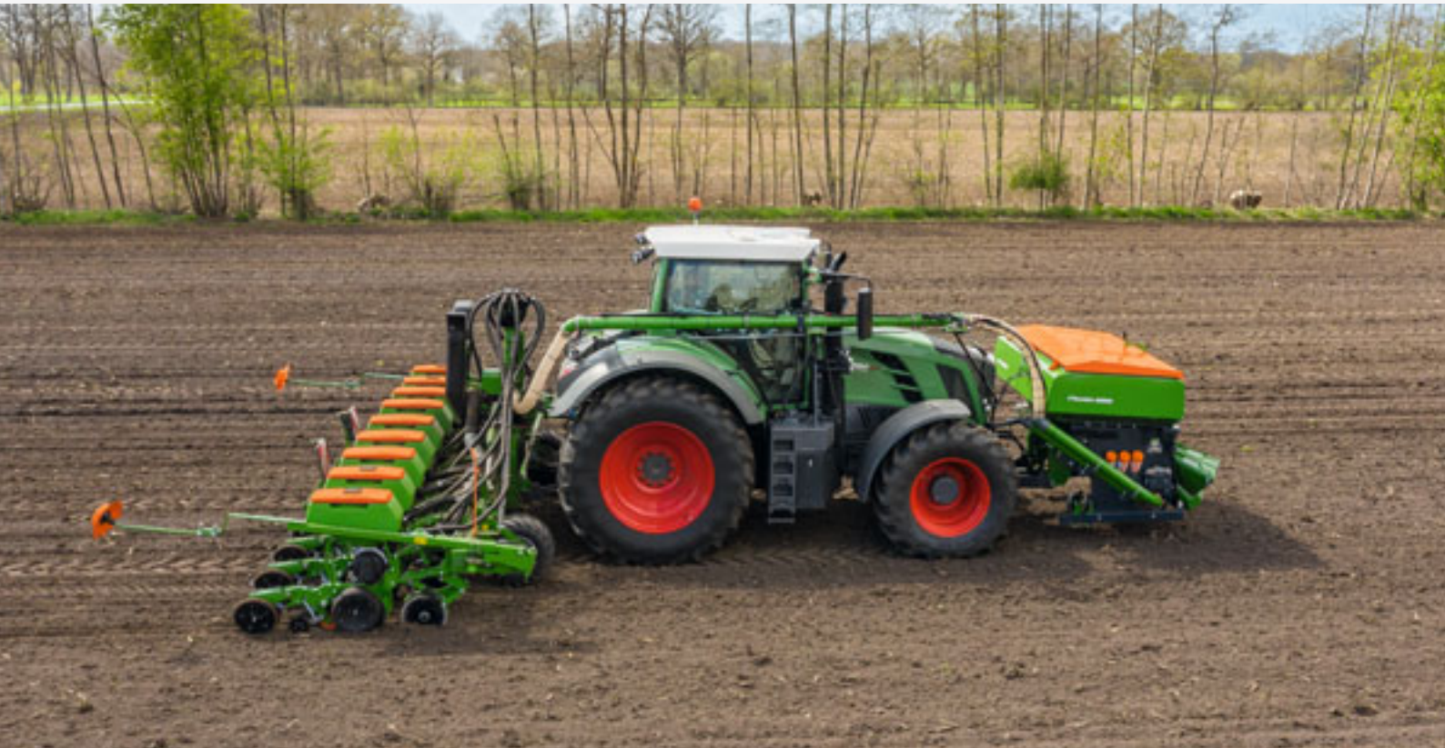
FTender 2200 mounted front hopper with Precea 6000-2FCC precision air seeder
