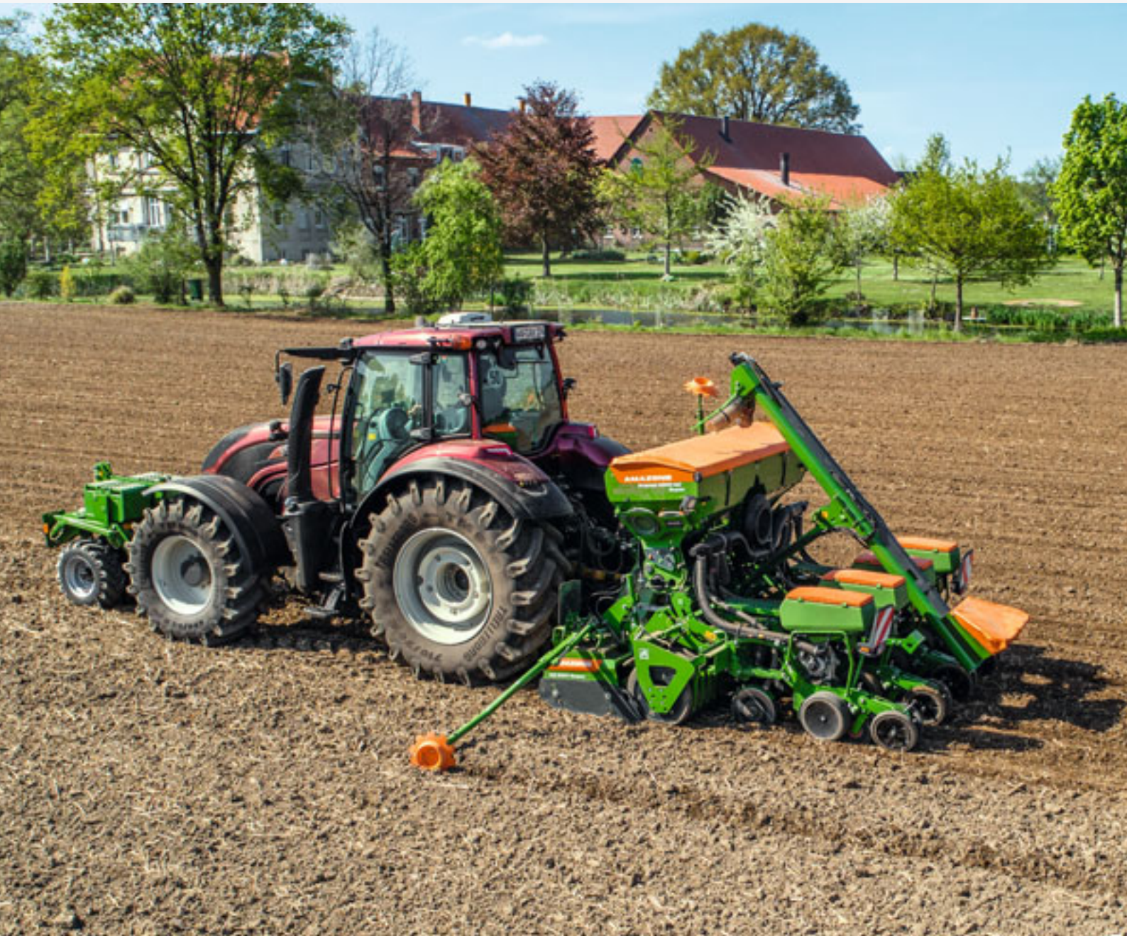
The Precea 3000-ACC with front packer in operation
