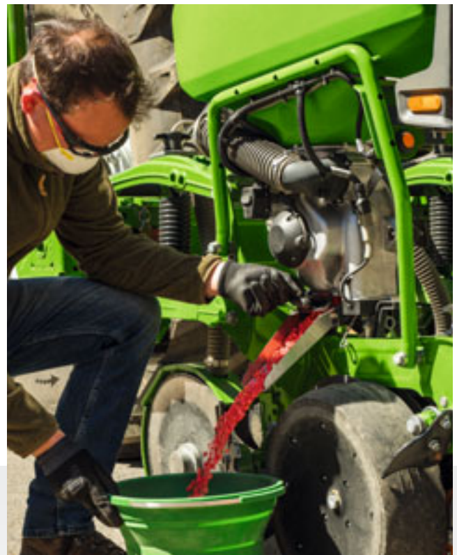
Emptying of residual amounts is particularly quick, clean and easy. And that can even be done from both sides.
