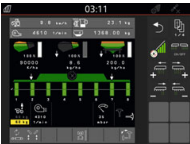
Clearly structured incorporation of the micro-granular applicator in the work menu of the terminal
