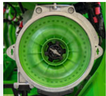
Singling disc in operation (without lid)
