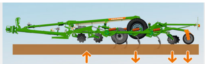
Operation with the tine element but without the disc element
