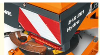
LED road traffic lights or conventional lighting
