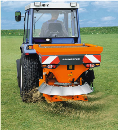
Application of sand
