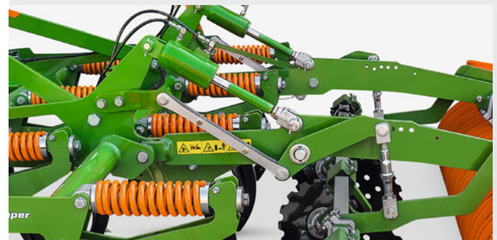
Automatic adjustment of the levelling unit
