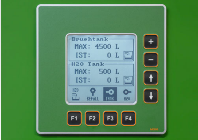
Entering of the desired fill levels for the spray liquid and fresh water tanks via the TwinTerminal with Comfort-Pack 2
