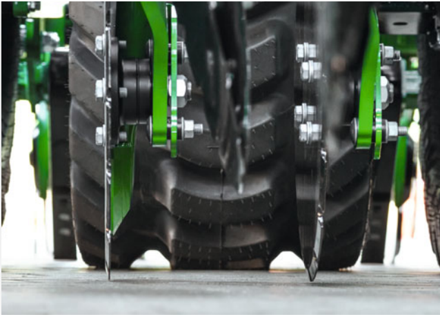
The FerTeC coulters are located in between the rows of the sowing coulters.
