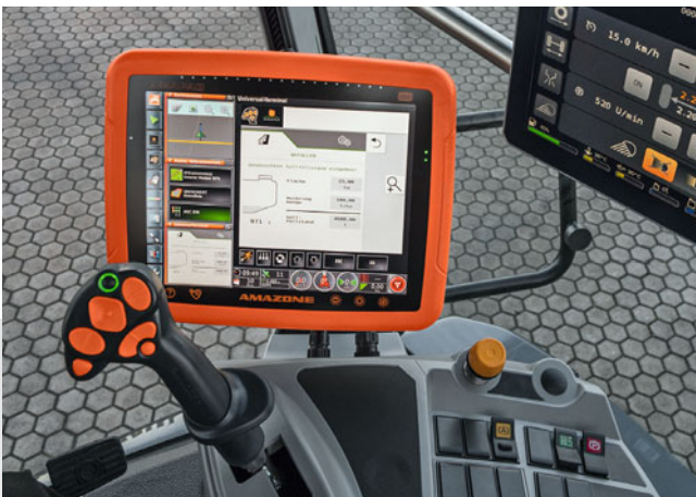
Entering of the desired fill level via the ISOBUS terminal
