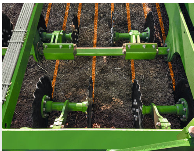
Cultivation in strips via Minimum TillDisc corrugated discs
