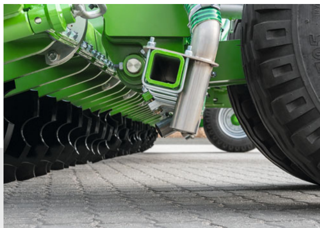
The liquid manure is delivered in front of the first disc row.
