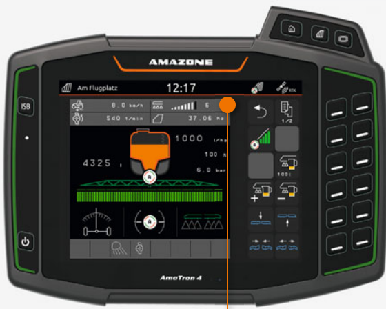
Display of the HighFlow + output capacity in the AmaTron 4 ISOBUS terminal
