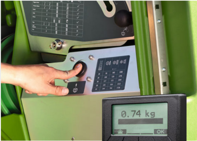
Calibration via calibration button or via TwinTerminal
