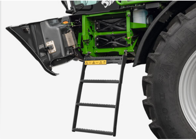
Dust-proof storage compartment under the access ladder
