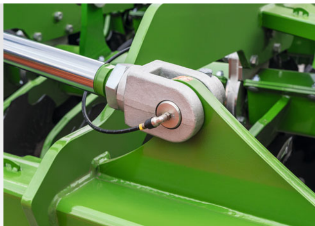
Additional greasing points on the fold points
