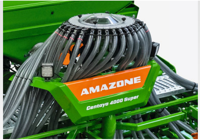
Segmented distributor head with electric half-side shut-off
