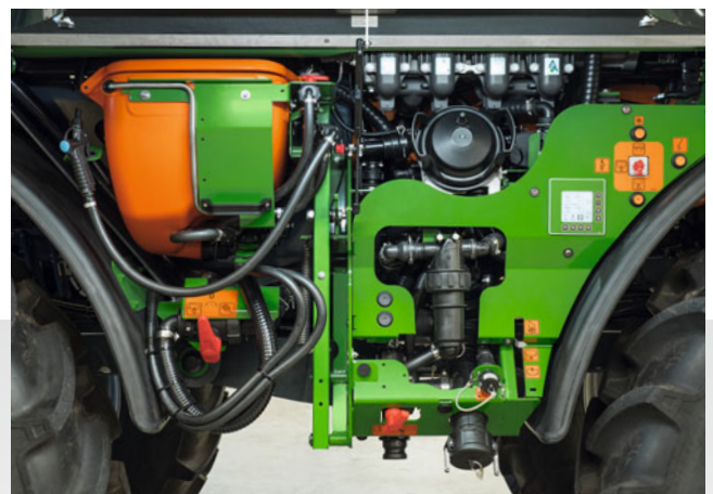
SmartCenter operator station with induction bowl and well laid-out valve chest
