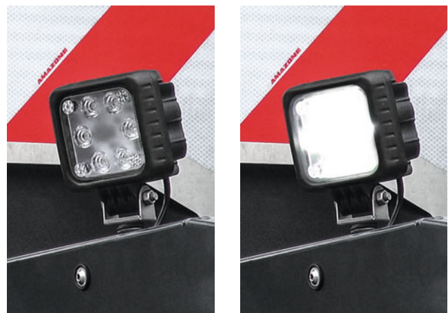
The working light kit informs the driver of the filling vehicle via flashing signals as to the quantity filled in.
