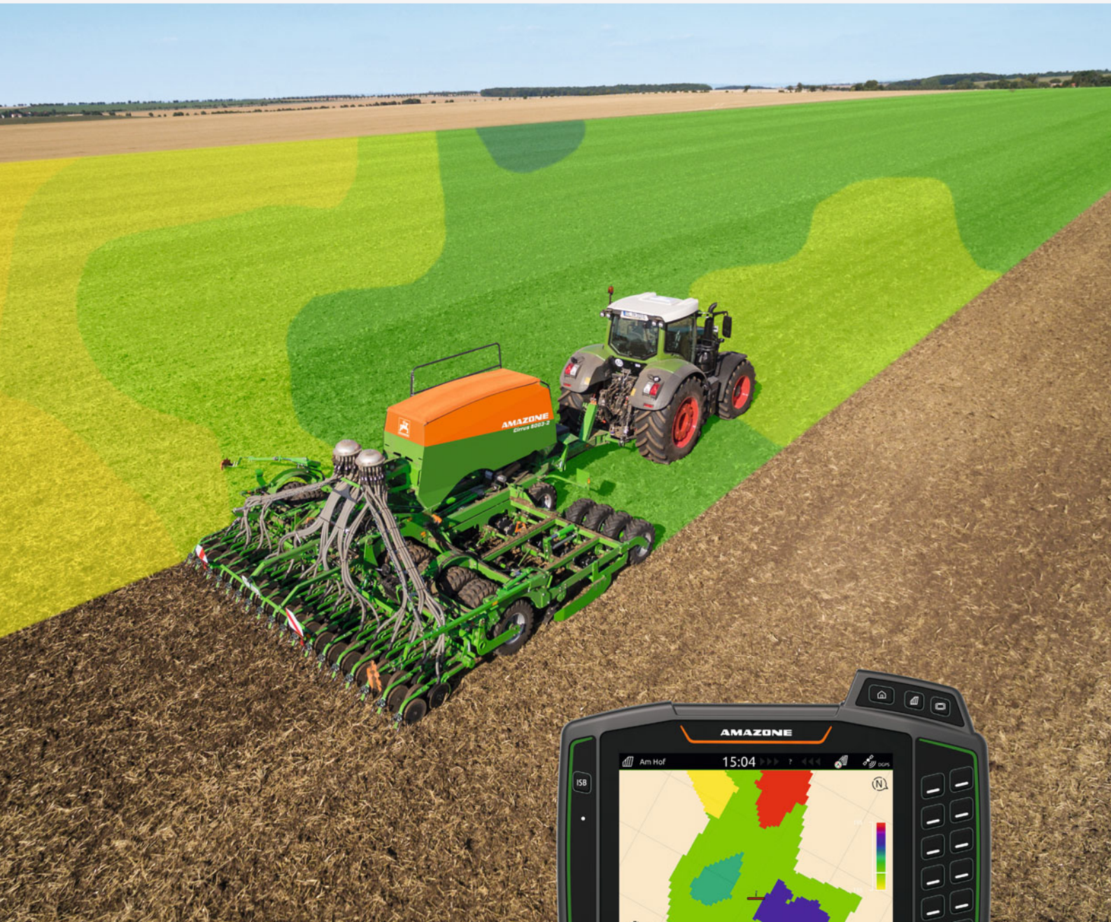
Part-area, site specific adjustment of the coulters pressure
