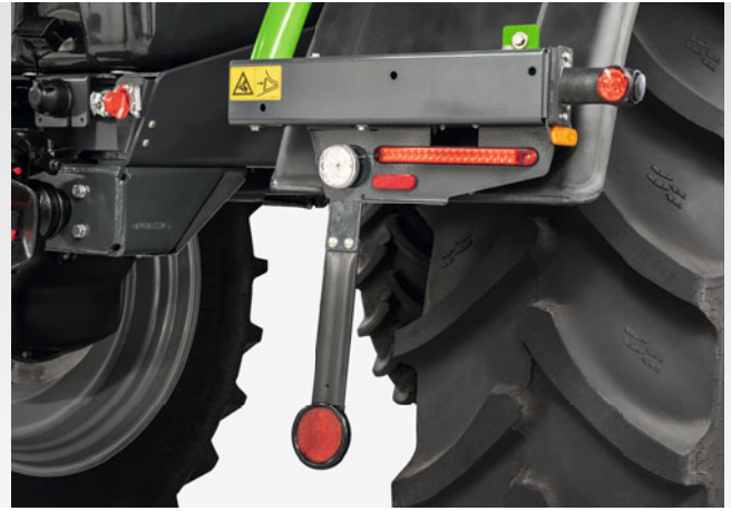
New LED rear road lighting
