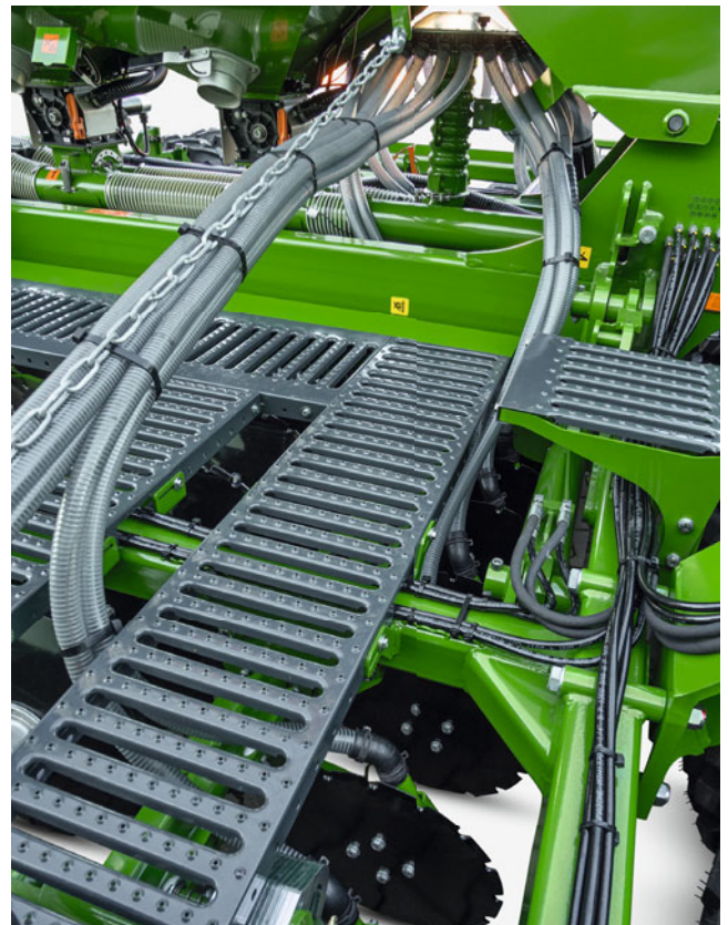
Tidy routing of the conveying hoses to the FerTeC coulters
