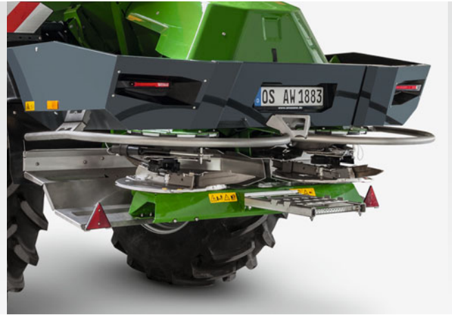
ZG-TS 01 features the AMAZONE TS spreading system
