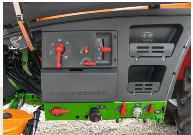
Standard Pack with manually operated valves
