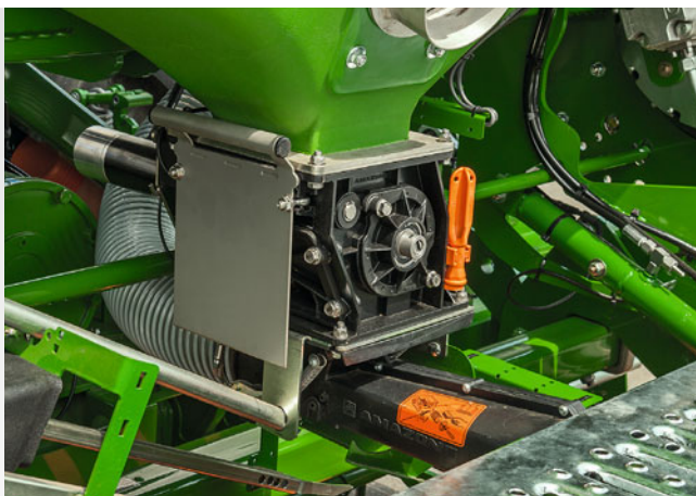
Electric metering drive via AmaDrill 2
