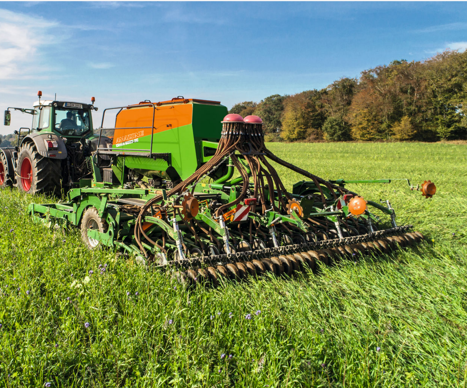
Cirrus 6003-2C with Minimum TillDisc – sowing cereals into an established catch crop
