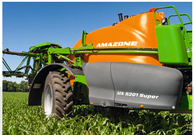
The new steering axle with 28 degree steering angle
